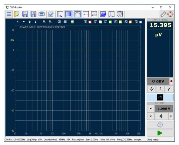
You can click on the marker  $\blacksquare$  button and inspect the amplitude of the measured signal: you should obtain a reading around 0dBV, this is the correct output level of the LogChirp signal with the generator output set to 1V.
