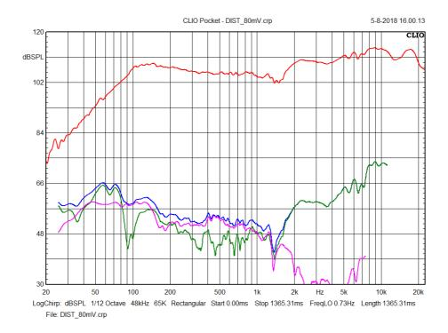
The level of the harmonic components can be very low, if the system is linear the IR of the harmonic components tend to sink into the measurement noise, which is basically the environmental noise. Thus a short measurement distance is beneficial also in this respect.
