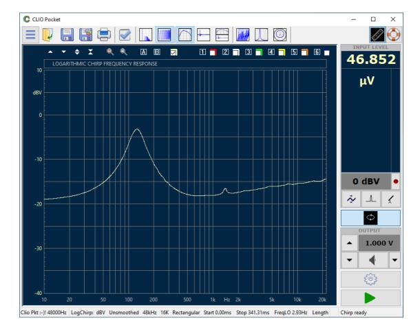
Actually this is not an Impedance Curve, but a Frequency Response showing the log scaled voltage division of CLIO's output impedance with the loudspeaker's input impedance. Open the LogChirp Settings  $\textcircled{}^{\textcircled{}}$  and change both Size to 65536 and Units to Ohm.
