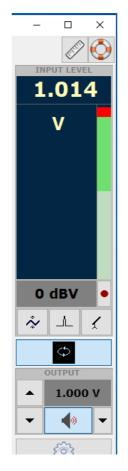
If everything is OK you should obtain a reading of circa 1V, variable between a minimum of 0.95V and a maximum of 1.05V, which is the mean output level of a sinusoidal signal when the system is not calibrated.
