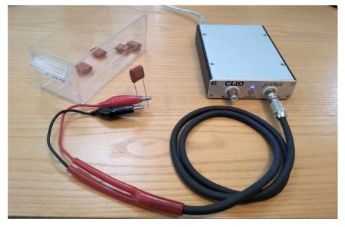
Pressing the  $\blacktriangleright$  arrow you should see a real time measurement of the component value.
