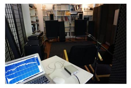
We are going to analyze the explosion of the balloon, which will give us a measure of the impulse response of our room. Open the FFT Option dialog and uncheck the RTA box, set the Event Trigger to Enable and One Shot, and input -5ms into the Delay edit box.
