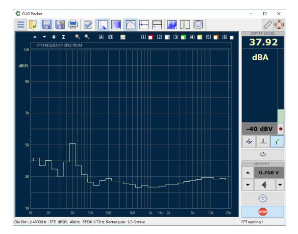
Before proceeding further, open again the Meter Options dialog and select Integration Impulse and Weighting Filter None, thus preparing for the next reading of the loudspeaker.
