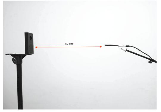
We should start by pairing the loudspeaker to the computer. Once the device is 4 ENJOY CLIO POCKET 75 paired and seen as a sound output device from the computer we can open CLIO Pocket software and check Enable Audio Device Playback Stream under CLIO Pocket Options–Device. Finally select the Bluetooth device under the Play Device list items.
