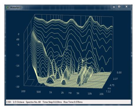
The CSD is a set of spectra calculated from progressively shorter sections of the measured impulse response. The idea is that by cutting the head of the impulse response, then the spectral analysis will reveal the frequency components that "holds" in the time response.
