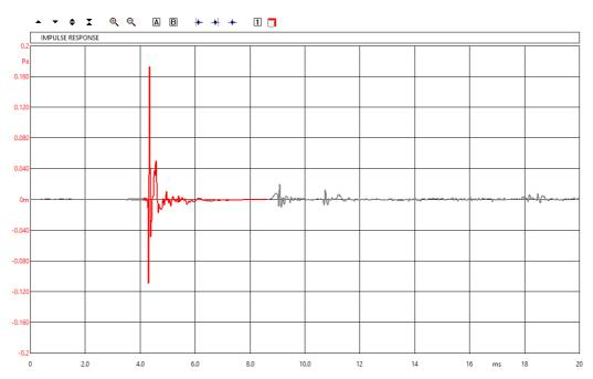
In this case there is only one overlay. It is also possible to **select** a portion of the main curve by means of three particular buttons. The selected portion of the main curve is identified by a **start** and **stop** point and is drawn in a different color from the unselected portion.
