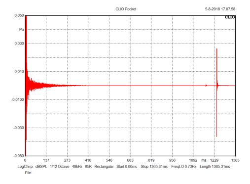
The harmonic distortion components impulse responses are clearly visible in the tail of the measured IR.
