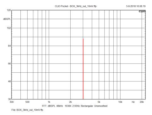
We then increment the driving level at 1 dB steps. As soon as the system starts to go over its linear range, a set of harmonic components of the input tone will appear at the output.
