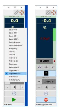
In this mode the multimeter shows the deviation from a reference value. The reference value can be set directly from the multimeter by clicking on the current reading, in our case 1.006 uF or the value can be set from the CLIO Pocket Options under the Meter tab:
