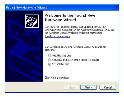
The wizard will direct you while installing the two drivers needed. You should *Install from a specific location* and point to the driver folder for XP on the CD (usually  $\$  Windows $\$ Driver $\$ XP) and then answer **Continue Anyway** to the prompt about Windows Logo testing.
