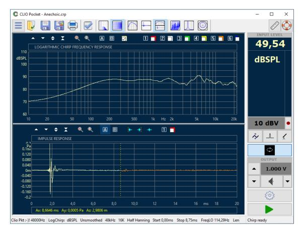
In the status bar, information regarding the measurements and its processing are reported. With the stop window set at 8.75ms and an impulse arrival time of 1.8ms the low frequency reliability limit is around 150 Hz. We did not set the Start Window, because it does not change the Frequency Response. If you are interested in anechoic responses it is unlikely you need a bigger measurement size than 16k, but for room acoustics 64k is advisable.
