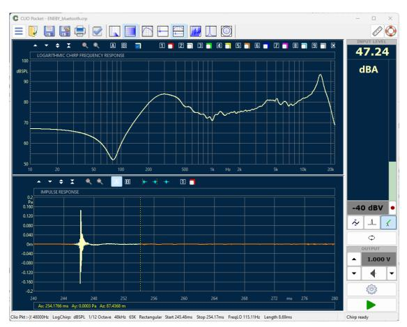
From the LogChirp measurement we can also evaluate the distortion:
